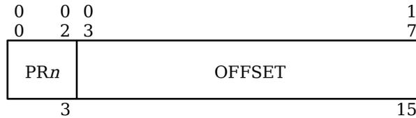
**Figure 6-7. Format of Instruction Word ADDRESS When Bit 29 = 1**
