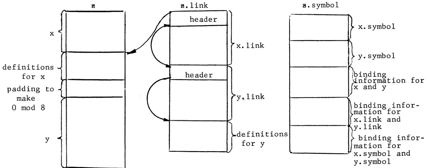
The binder copies `input_name1` and `input_name1.link` into `output_name` and `output_name.link` and appends words of zeroes as padding in order to make each component segment have length 0 modulo 8. `input_name1.symbol` is copied into `output_name.symbol` up to the start of the binding information; it also is padded with zeroes to make it have length 0 modulo 8.
