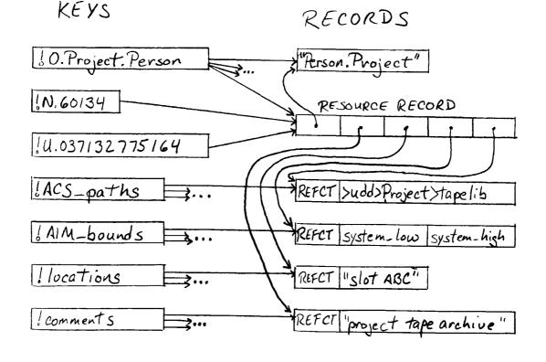
Figure I: Sample Chaining for Tape 60134
